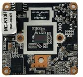
The MC-K10H module is a camera module designed for the timely detection and alarm signaling of smoke and flames, suitable for both indoor and outdoor environments. Its smoke and flame detection algorithms can identify smoke and flame regions within dynamic video streams. After multi-frame fusion calculations, it can output alarm information for smoke and flames.
